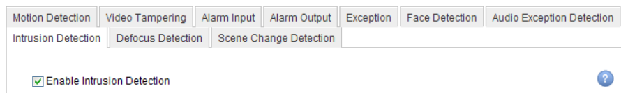
Figure 6-12 Setting Intrusion Detection on IP Camera
